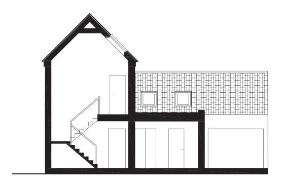
Cross-section through the staircase and the entrance area. In the background the kitchen windows in the roof and the garage door.
